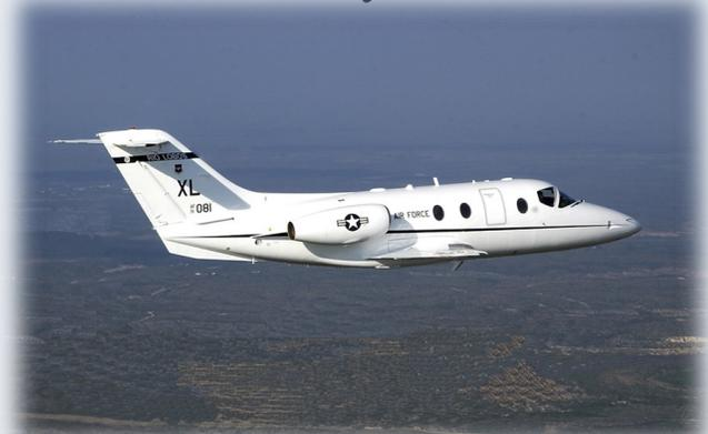
The T-1A Jayhawk is a medium-range, twin-engine jet trainer used in the advanced phase of Specialized Undergraduate Pilot Training for students selected to fly airlift or tanker aircraft. It is also used to support navigator training for the U.S. Air Force, Navy, Marine Corps and international services.
